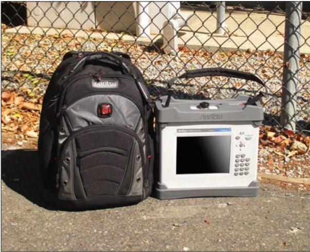
PIM Master MW82119A 40 Watts, Battery-operated
