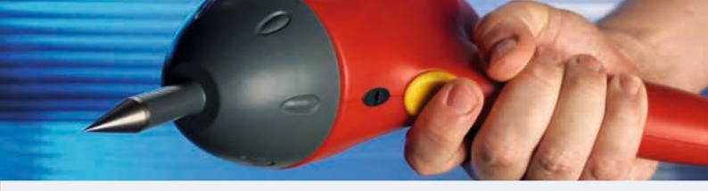
**The simulator contains a threshold detector** to eliminate faulty discharge counts over its wide operating voltage range and applications. Only valid HV discharges are indicated. When discharges are detected, the counter or preset counter is incremented or decremented respectively – a particularly useful feature for long test runs. The detection feature can be switched off when testing EUT's with non-conductive surfaces, such as plastic housings.
