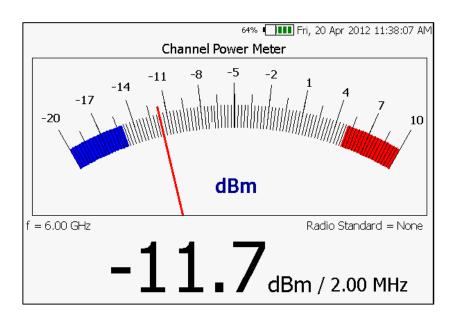
Built-in Power Meter (also known as Channel Power Meter) uses the SA input connector to make quick and simple power measurements over a selectable frequency band. A power sensor is NOT required.
