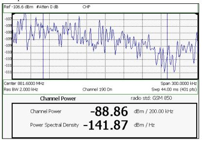
Channel Power measurement; Chan 190 Downlink; GSM850 Radio Standard
