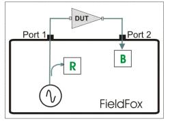
2-Port Transmission measurement of an amplifier
