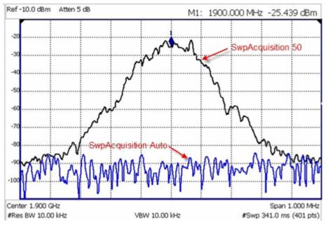
A GSM signal in a framed data format; timeslot zero ON; all others OFF; PRF = 218Hz, Duty Cycle = 12.5%. The pulsed signal becomes visible on every sweep update with SwpAcquisition = 50.
