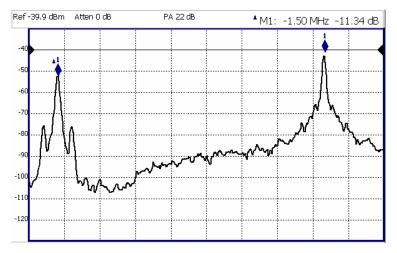
A Delta marker and its associated reference marker. The marker readout shows the difference between the two markers in frequency and amplitude.
