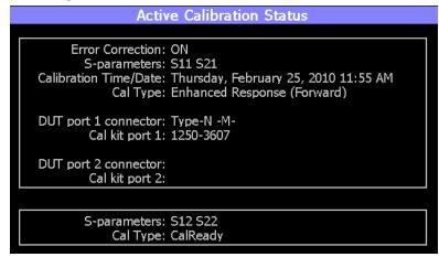
The top box shows the properties of the current calibration that you performed and the displayed S-parameters that it is correcting.
