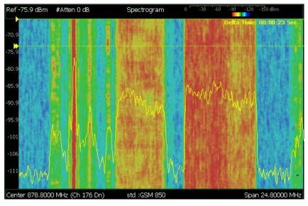
Spectrogram display- Overlay view- with time markers 23 seconds apart.
