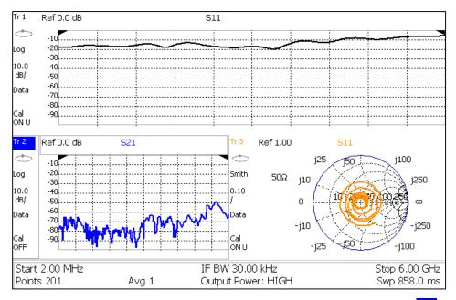
An x3H configuration. Tr2 is the ACTIVE trace as indicated by the highlighted Tr 2
