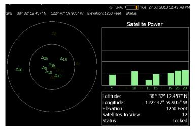
• The left portion of the screen shows satellites and the corresponding number on the adjacent Satellite Power chart.
