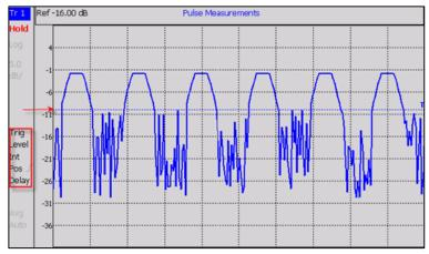
Trig Level = -10 dBm, Trig Type (Int), Pos Slope (/), Delay
