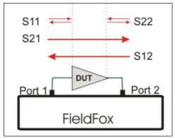
The FieldFox automatically switches the internal source and receivers to make both forward and reverse measurements. Therefore, the FieldFox can measure all four S-parameters with a single connection.
