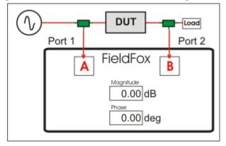
B/A Transmission measurement with external source
