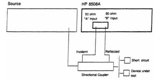
Typical 8508A measurement configuration -as shown in the 8508A manual.
