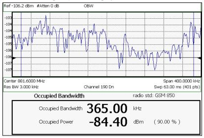
OBW measurement; Chan 190 Downlink; GSM850 Radio Standard
