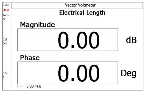
Display for the 1-Port Cable Trimming measurement
