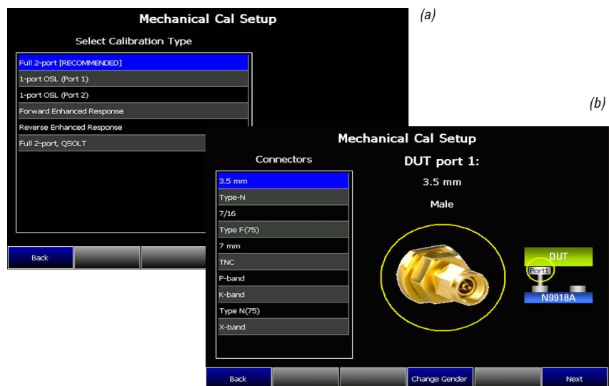
Figure 17. FieldFox Calibration (Cal) Wizard display screens showing (a) selecting the calibration type and (b) selecting the DUT connector type
