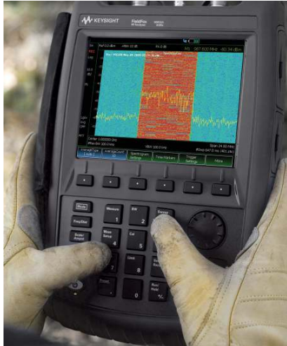
RF spectrum monitoring aided by spectrogram recording
