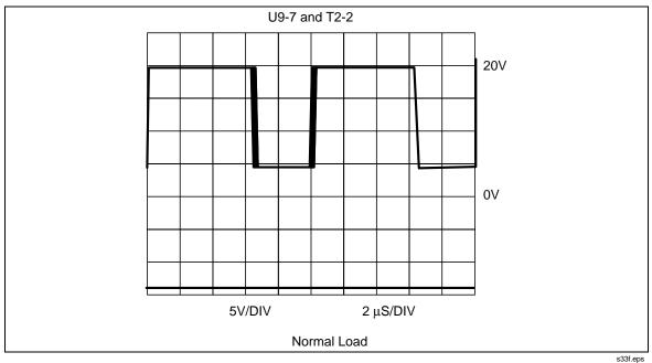
Figure 5A-2. 5-Volt Switching Supply (2635A)
