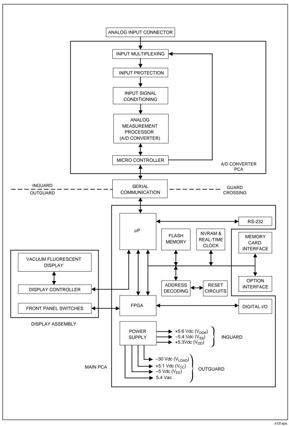
Figure 2A-2. Overall Functional Block Diagram (2635A)
