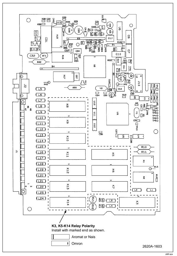
Figure 6-6. A3 A/D Converter PCA
