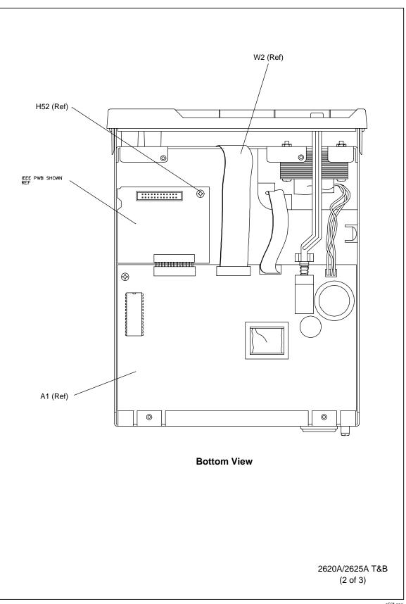
Figure 6-1. 2620A/2625A Final Assembly (cont)
