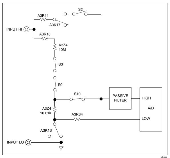
Figure 2-4. DC Volts 300V Range Simplified Schematic
