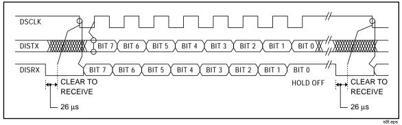
Figure 2-8. Command Byte Transfer Waveforms
