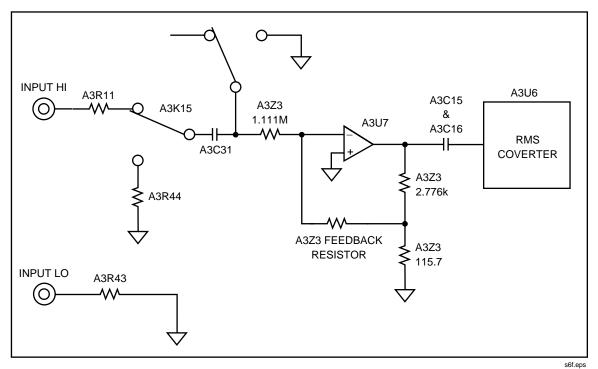
Figure 2-6. AC Buffer Simplified Schematic
