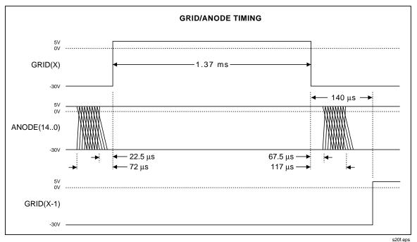
Figure 2A-10. Grid-Anode Timing Relationships (2635A)
