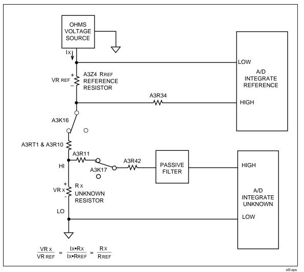
Figure 2-5. Ohms Simplified Schematic
