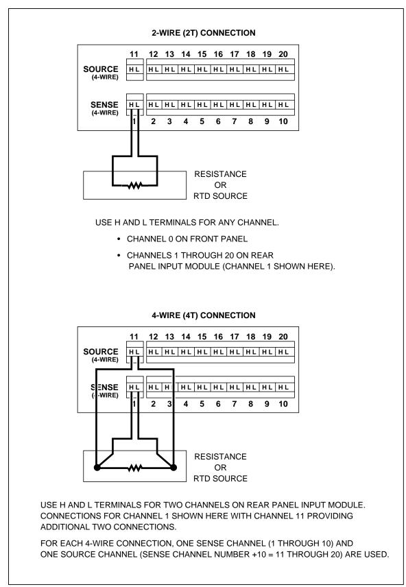
Figure 4-2. 2T and 4T Connections
