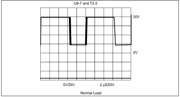
Figure 5-2. 5-Volt Switching Supply
