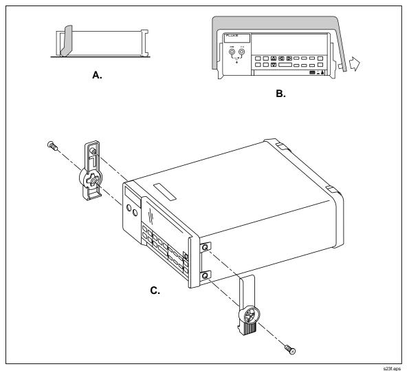
Figure 3-3. Removing the Handle and Handle Mounting Brackets
