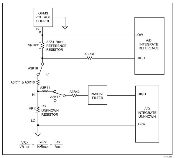
Figure 2A-5. Ohms Simplified Schematic (2635A)
