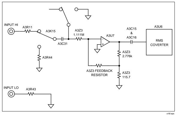
Figure 2A-6. AC Buffer Simplified Schematic (2635A)
