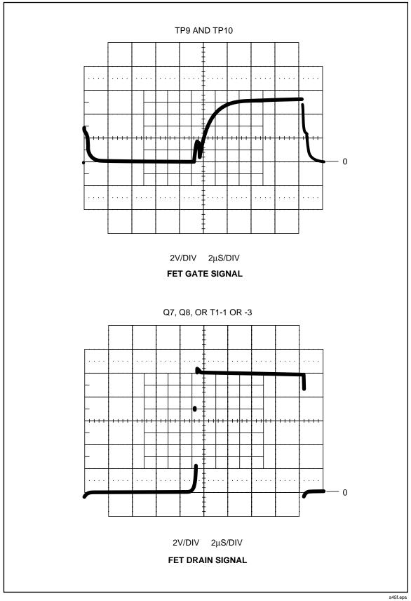
Figure 5A-3. Inverter FET Drive Signals (2635A)
