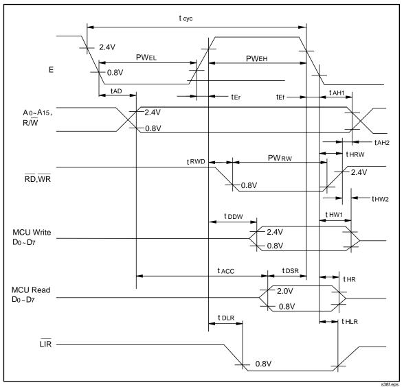
Figure 5-7. Microprocessor Timing
