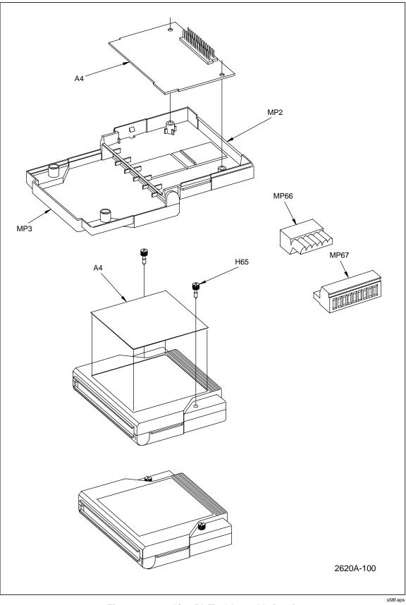
Figure 6-1. 2620A/2625A Final Assembly (cont)
