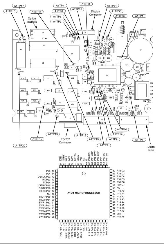
Figure 5-1. Test Point Locator, Main PCA (A1)
