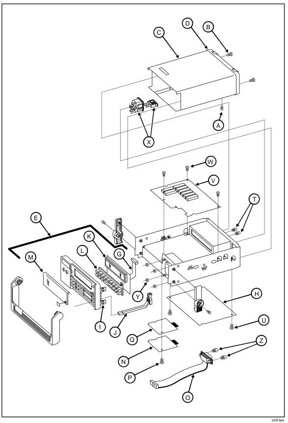
Figure 3-4. 2620A and 2625A Assembly Details
