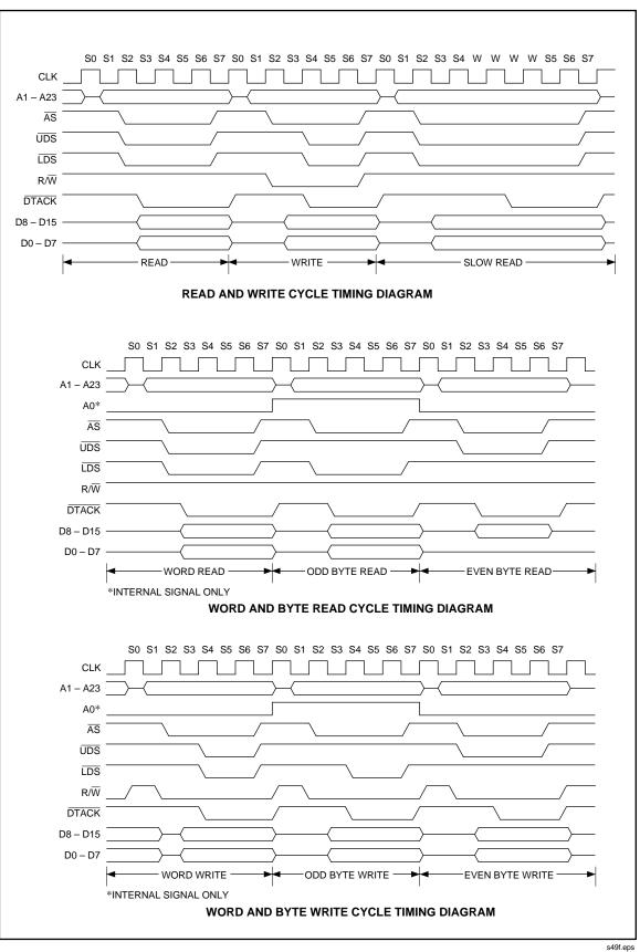
Figure 5A-7. Microprocessor Timing (2635A)
