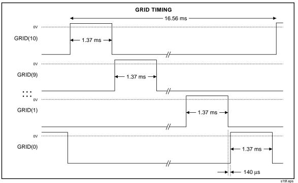
Figure 2A-9. Grid Control Signal Timing (2635A)
