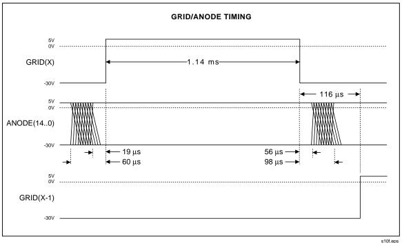
Figure 2-10. Grid-Anode Timing Relationships
