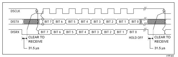
Figure 2A-8. Command Byte Transfer Waveforms (2635A)
