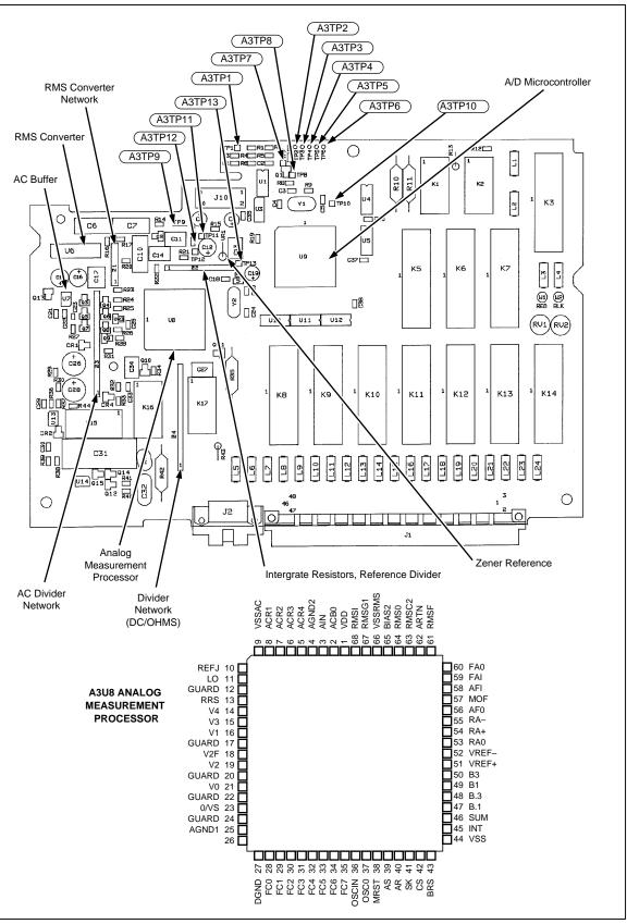
Figure 5-4. Test Points, A/D Converter PCA (A3, A3U9)
