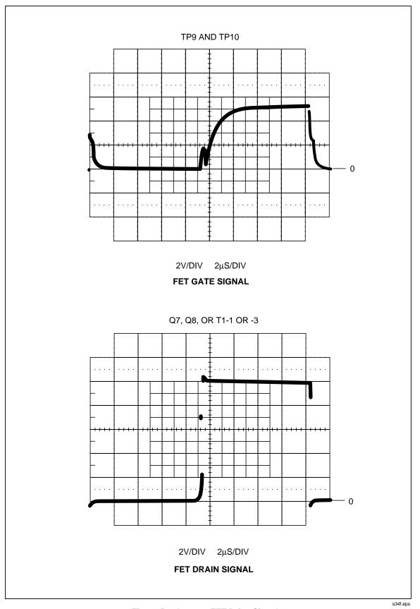
Figure 5-3. Inverter FET Drive Signals
