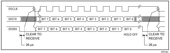
Figure 5-9. Display Controller to Microprocessor Signals
