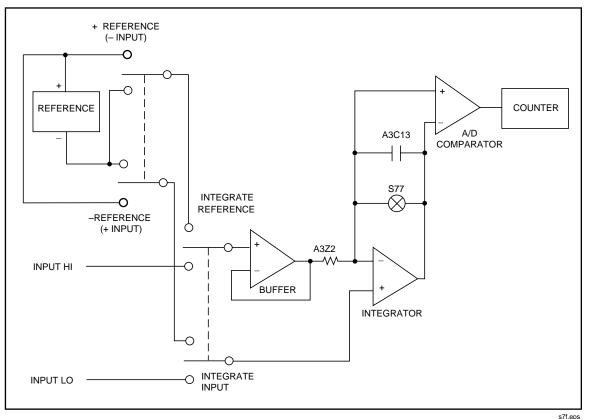
Figure 2-7. A/D Converter Simplified Schematic
