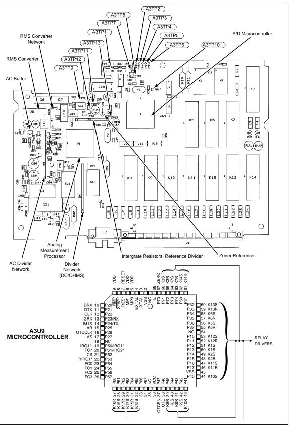
Figure 5-5. Test Points, A/D Converter PCA (A3, A3U9)
