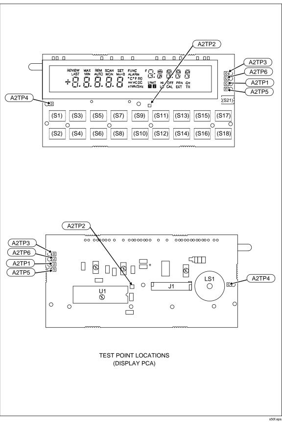
Figure 5A-8. Test Points, Display PCA (A2) (2635A)
