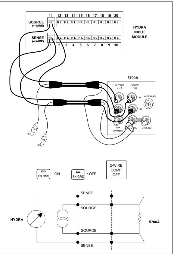
Figure 4-6. 4-Terminal Connections to the 5700A
