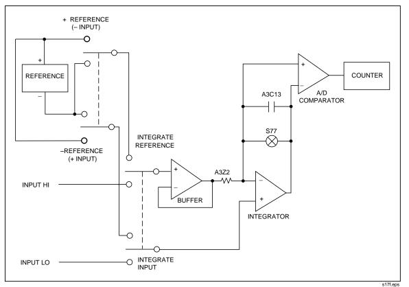
Figure 2A-7. A/D Converter Simplified Schematic (2635A)
