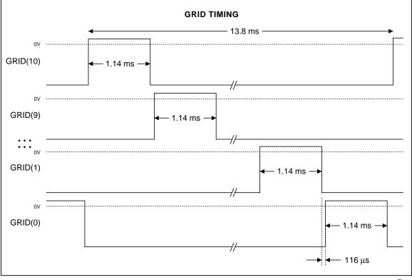
Figure 2-9. Grid Control Signal Timing
