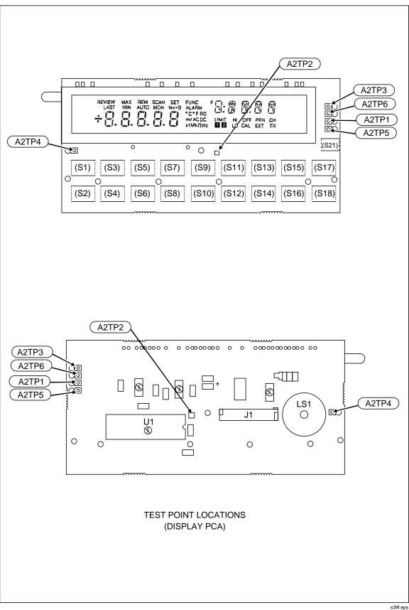
Figure 5-8. Test Points, Display PCA (A2)
