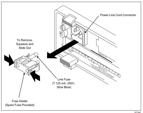
Figure 3-1. Replacing the Line Fuse
