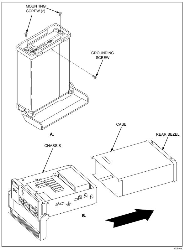
Figure 3-2. Removing the Case
