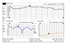
The above image shows a 3-trace configuration. **Tr1** is the **ACTIVE** trace as indicated by the highlighted **Tr1** annotation in the upper left corner.
