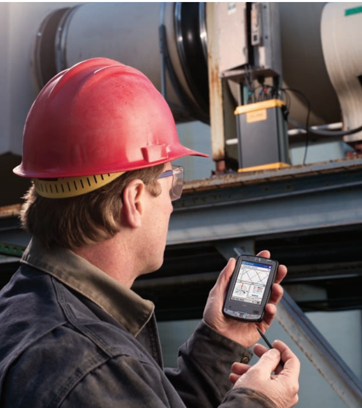
Checking data during recording with the wireless PDA feature of the FLuke 1750 Power Recorder.
