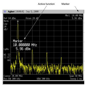
Figure 3-3 A Marker on the 10 MHz Peak
