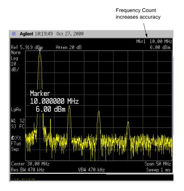
Figure 3-6 Using Marker Counter
