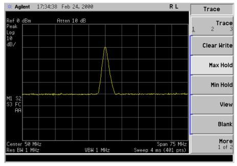
6. Activate trace 2 and put it into minimum hold by pressing **Trace (2)**, **Min Hold**. Your analyzer display should look similar to Figure 4-4.
