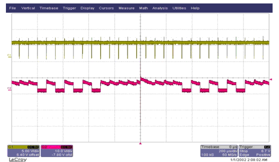
Fig. 18 Output after a discharge of a 15kV at a distance of 0.3m
