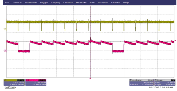
Fig. 14 Output after a discharge of a 15kV at a distance of 0.9m
