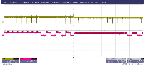
Fig. 19 Output after a discharge of a 15kV at the 555 timer output
