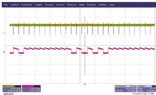
Fig. 17 Output after a discharge of a 15kV at a distance of 0.3m
