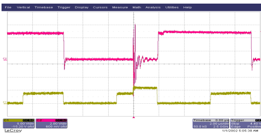
Fig. 5 Output when data is triggered at low and clock is triggered at high.
