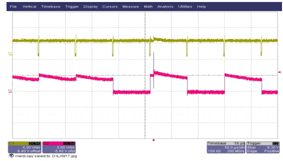
Fig. 16 Output after a discharge of a 15kV at a distance of 0.5m
