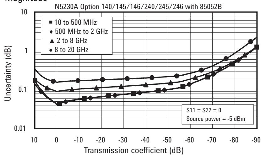
1. From 300 kHz to 10 MHz, performance is characterized as "typical". To generate these typical values, please download our free Uncertainty Calculator from [www.agilent.com/find/na\\_calculator](http://www.agilent.com/find/na_calculator).
