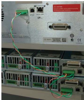
Figure 3b. Multiple mainframe wiring
