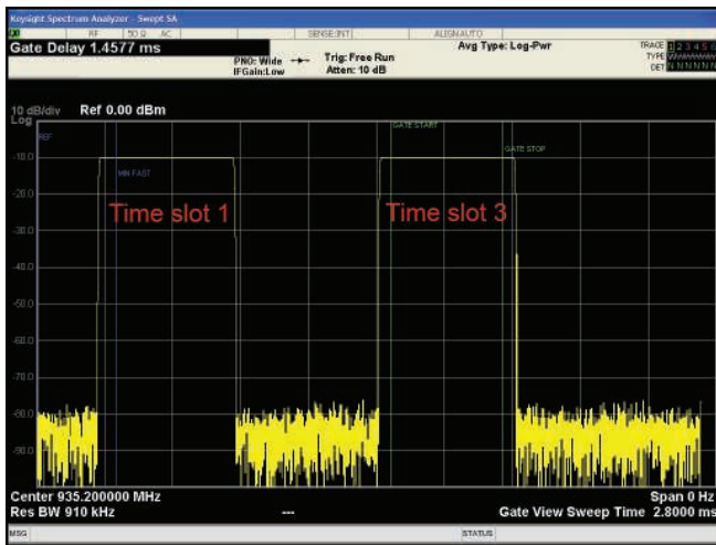
Figure 2-38. Time gating is used to look at the spectrum of the GSM time slot 3.
