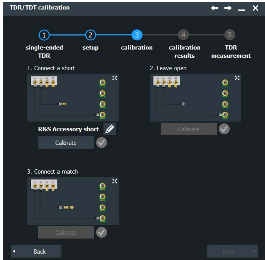
Figure 16-3: Calibration of single-ended TDR/TDT
