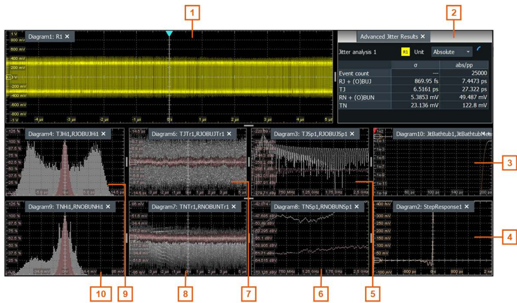
Figure 18-5: Advanced jitter and noise analysis results display
