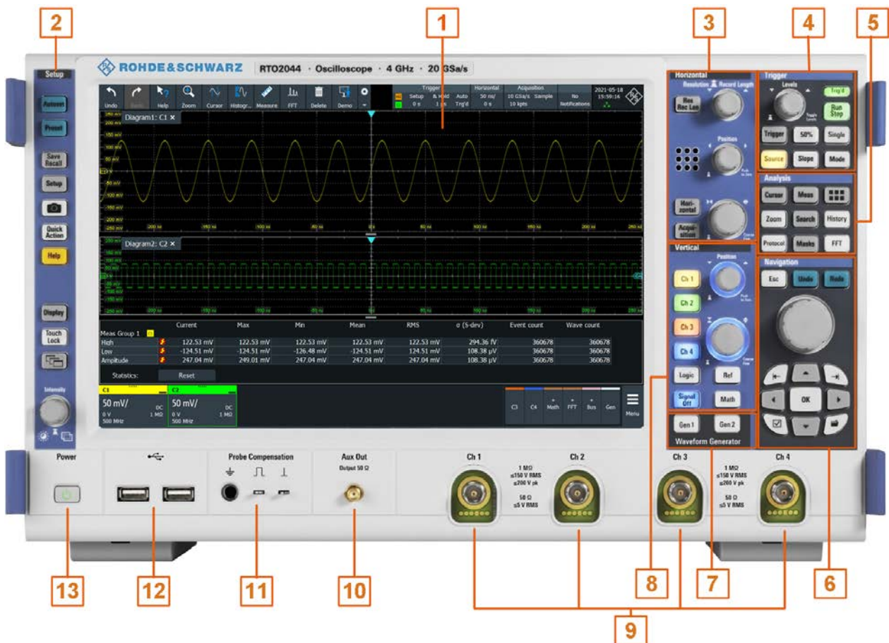
Figure 3-1: Front panel of R&S RTO2044 with 4 input channels
