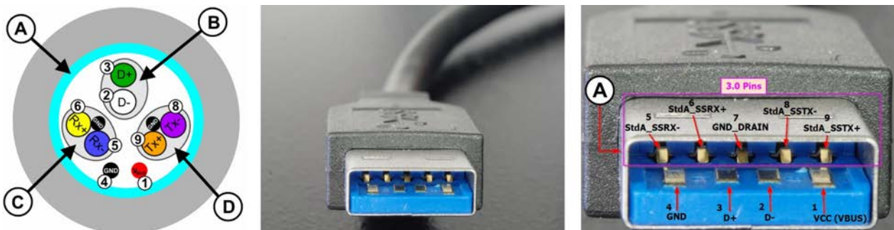
Figure 13-39: USB 3.1 cable cross-section and Standard-A plug - backward compatible with USB 2.0
