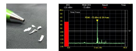
Dynamic testing identifies loose metal-to-metal connections as well as contact surface defects that might cause arcing at higher power levels. Without dynamic testing these defects could go unnoticed until activated by wind loading, tower vibration or stresses caused by temperature changes.
