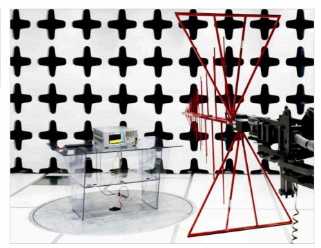
Electromagnetic compatibility (EMC) testing requires detailed and exacting methodologies to ensure that all emissions are accurately measured. Long test times impact test facility availability and reduce the number of devices that can be certified—capping the amount of revenue a testing service can generate or the number of new devices a company with internal test capabilities can introduce without the cost of third party testing.
