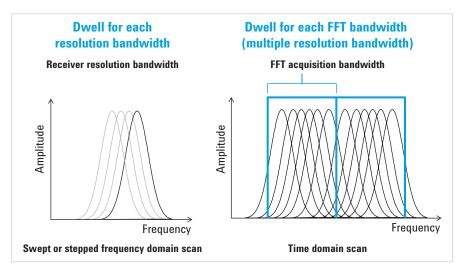
Figure 1. Comparison of resolution and FFT acquisition bandwidths
