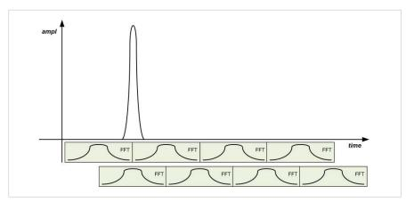
Figure 2b. Measurements made with FFTs highly overlapped in the time domain increase probability of intercept and minimize amplitude measurement scalloping
