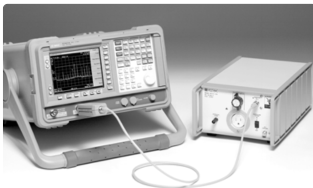
Use the EMC analyzer with the 84115EM-11967D LISN device to test for conducted emissions.
