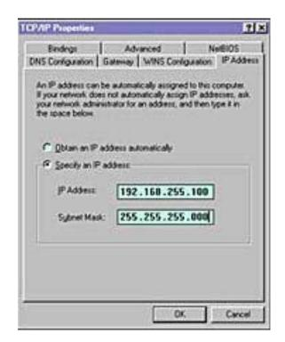
At this point, the PC's network address is 192.168.255.100. The Astro-Med Data Acquisition Recorder ships as address 192.168.255.1. To verify network setup and connections, use the Ping command.
