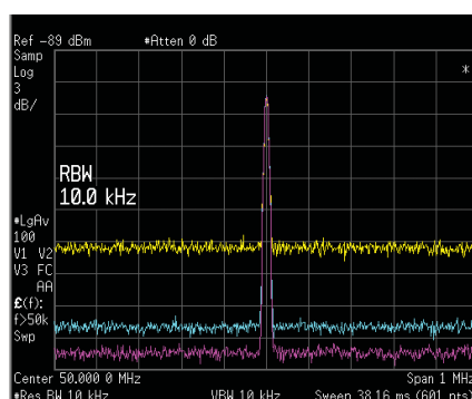
Figure 10. Signal after minimizing resolution bandwidth, input attenuator and using logarithmic power averaging
