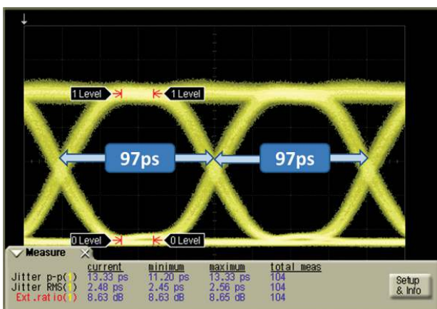
Figure 13. Measurement of the same multiplexer using Rapid Eye, demonstrating more complete characterization of the eye and the same bit periods.
