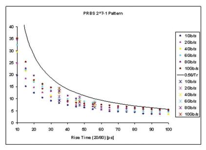
Figure 6: The amount of bandwidth (in GHz) required to contain 99.9% of the signal power of a  $2^7-1$  PRBS pattern
