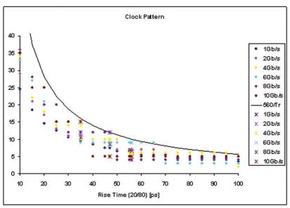
Figure 5: The amount of bandwidth (in GHz) required to contain 99.9% of the signal power of a clock pattern 0.56/Edge Speed
