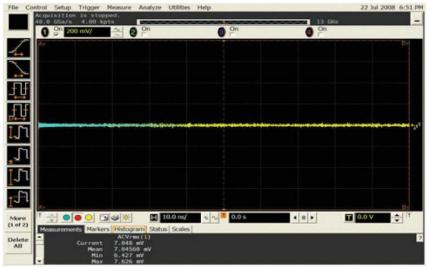
Figure 1: Measuring the noise floor at 200 mV/div
