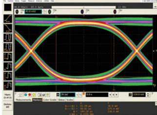
Figure 4: PCIe® Gen II 60-pS rise time captured 8 GHz
