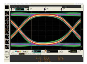
Figure 3: PCI Express® Gen II signal captured at 13 G with 60 pS rise time
