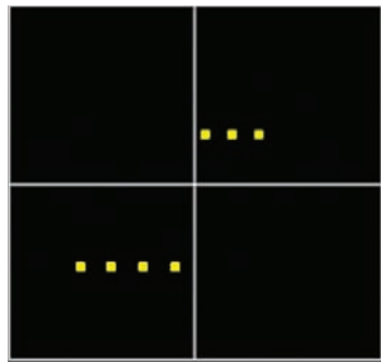
Figure 27. Waveform where the sample rate yields seven data points per period
