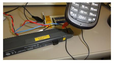
Figure 4-2. A simple way to measure a current with an oscilloscope is to use a clamp-on type current probe such as Keysight's 1147B or N2893A.
