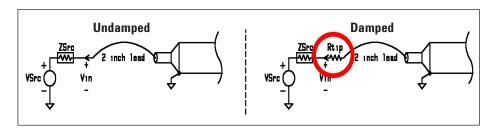
Figure 8-2. With a properly damped probe input, the loading/input impedance will never drop below the value of the damping resistor.  $\frac{1}{2}$
