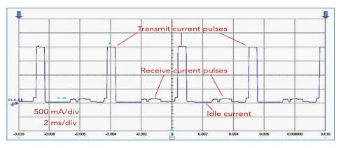
Figure 4-1. The current drain measured on a GSM cell phone when making a call.
