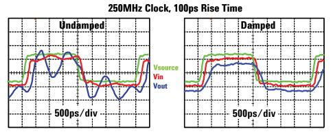
Figure 8-3. As the speeds in your design increase, you may notice more overshoot, ringing and other perturbations. Overcome the resonance formed by the connection of a probe by adding a damp resistor to your probe tip.
