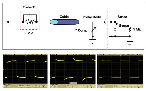
Figure 3-2. Compensation adjustment corresponds to the flat square wave
