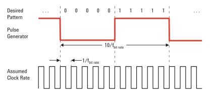
Figure 12: Square wave from pulse generator simulating 0000011111 pattern
