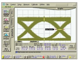
Figure 28: RIN OMA Result for an Externally Modulated Laser (EML)
