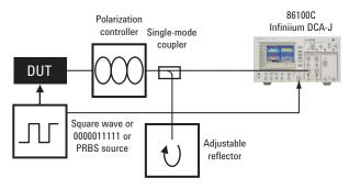
Figure 4: Agilent 86100C Infiniium DCA-J based setup<sup>3</sup>
