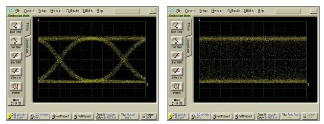
Figure 8: PRBS eye diagram in oscilloscope mode (left: triggered, right: free run)
