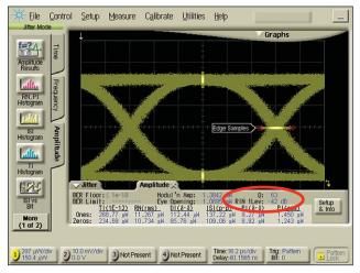
Figure 9: RIN "1' level result in jitter mode
