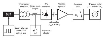
Figure 16: IEEE 802.3ae based setup for RIN OMA
