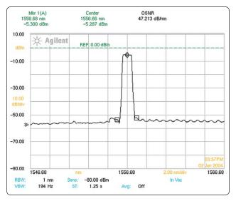
Figure 1: Distributed feedback (DFB) laser spectrum
