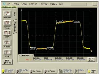
Figure 3: OMA measurement on a square-wave signal
