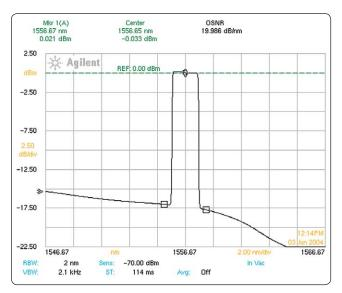
10 The 86146B has about 5 dB loss when operated as a tunable filter. It is recommended to verify the optical signal with a power meter and adjust the second attenuator before connecting the OSA's output with the DCA-J.
