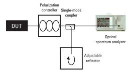
Figure 22: Optical spectrum analyzer setup
