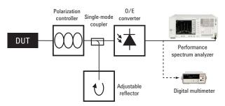
Figure 20: Electrical spectrum analyzer setup
