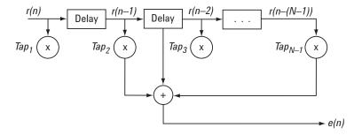
Figure 8: A shift register description of a linear feedforward equalizer.
