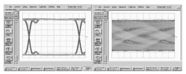
Figure 1: (a) A clean eye observed from the transmitter, (b) the same signal observed at the end of a substantial trace on FR4.
