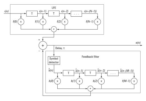
Figure 10: The DFE is a combination of two shift registers.
