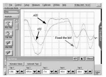
Figure 6: The received and equalized signals using the built in LFE on the Agilent DCA-J.
