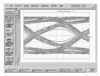
Figure 2: A signal with ample ISI illustrating the different trajectories of the bit transitions in a repeating pattern.
