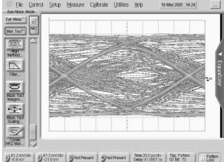
Figure 7: The received and equalized eye diagrams.
