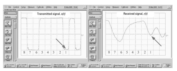
Figure 5: The same segment of a data signal before and after traversing a backplane. The red arrows indicate the bit studied in the text.
