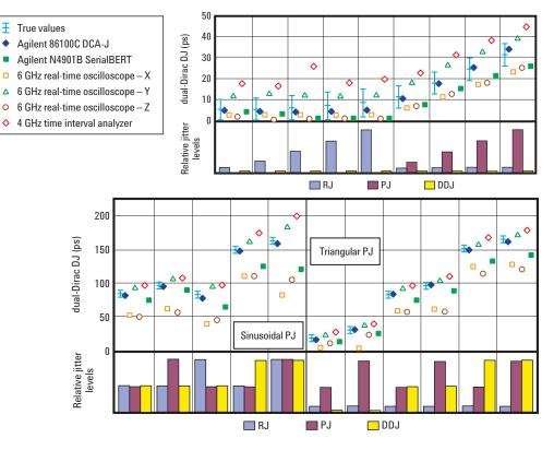
Figure 8: Measurements of the dual-Dirac DJ with jitter conditions. The jitter conditions (RJ, PJ, DDJ) of each measurement are indicated by the bar graph at the bottom. The true values of dual-Dirac DJ and the calibration uncertainties associated with them are indicated by the left-most, white, data point in each column.
