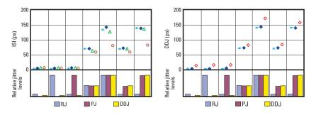
Figure 10: The (a) ISI and (b) DDJ measurements for an illustrative subset of conditions.
