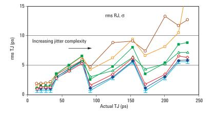
Figure 5: rms RJ measurements by the different test-sets vs the true value of  $TJ(10^{-12})$ . The true values of RJ are indicated by the white curve. The error bars on the true values indicate the calibration uncertainty in the calculation of the true values. The complexity of the jitter conditions for each measurement increases from left to right, as does the discord among the analyzers.
