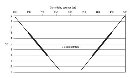
Figure 6: Graph of an applied RJ signal on a Q-scale. That the data is a straight line down to a value of Q less than 7 indicates Gaussian behavior down to BER less than  $10^{-12}$ .
