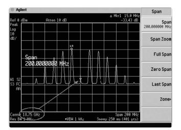
Figure 5: The Bessel null of the 15th harmonic.
