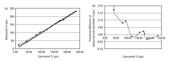
Figure 7: Comparison of  $TJ(10^{-12})$  calculated from the various RJ/DJ calibrations with measurements performed on a BERT. In (a) the measured TJ is plotted against the calculated values, the straight line would correspond to perfect agreement; in (b) the fractional difference between the calculated and measured values of TJ show agreement of better than 10% that can be accounted for by intrinsic uncertainties in the BERTscan technique.
