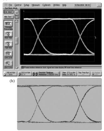
Figure 3: Comparison of the measured baseline eye diagram, (a), with the eye diagram calculated from the frequency response of the transmission path, time-averaged impulse response of the pattern generator on a PRBS7 and the observed baseline RJ.
