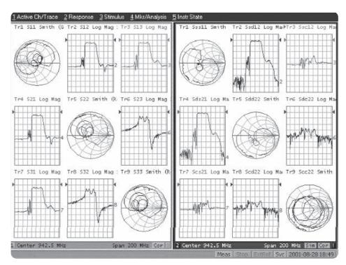
Figure 14. Single-ended and corresponding mixed-mode measurement parameters
