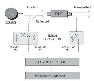
VNA hardware consists of a sweeping signal source (usually internal), a test set to separate forward and reverse test signals, and a multichannel, phase-coherent, highly sensitive receiver (figure 1). In the RF and microwave bands, typical measured parameters are referred to as S-parameters, and are also commonly used in computer-aided design models.
