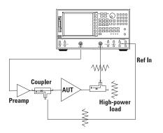
Figure 2. High-powered foward measurement configuration
