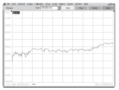
Figure 11. Measurement of load standard after calibration
