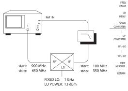
Figure 7A. Mixer measurement setup
